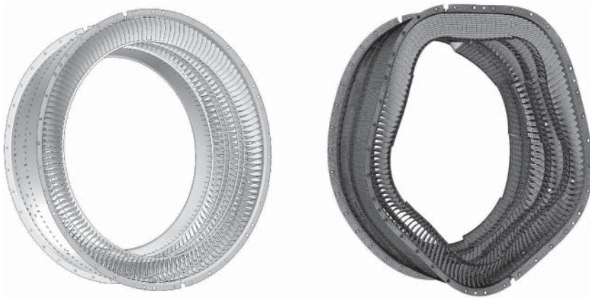
Figure 1 Finite element model of a stator section of aircraft engine. Source: Reproduced with permission from Techspace Aero – SAFRAN Group.
